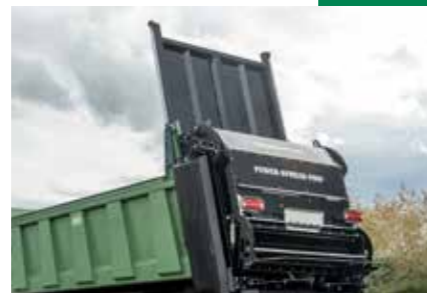
Storage wall Better utilization of loading volume and a perfect spreading pattern from the start
