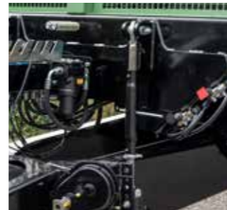
Coupling height adjustable via spindles
