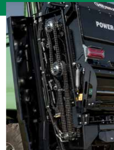
Chain drive of the lower milling drum with 1-inch duplex chain and the upper milling drum with 5/4-inch chain
