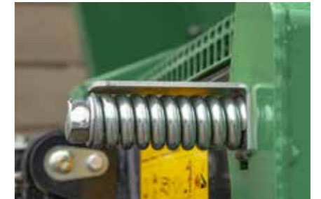
Chain tensioner spring-loaded with indicator on the front wall
