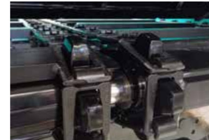
Chain strands with flat link chain instead of round steel chain (optional)
