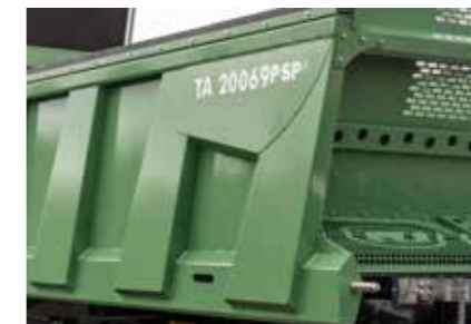
Stabilizer sidewalls bolted to the frame in two directions
