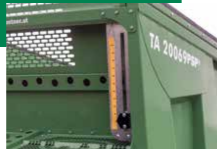
Storage wall display on the front wall with concealed cable guide, protecting against dirt buildup and malfunctions
