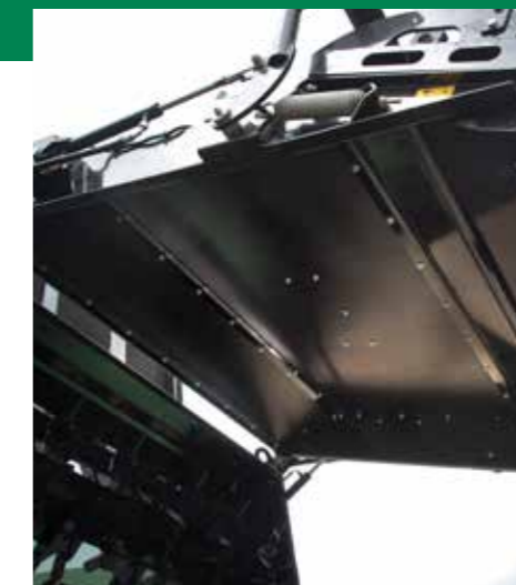
Hydraulic cover hood with plastic wear plates
