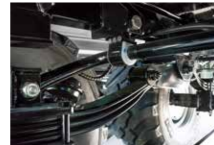
Suspension stabilizer highly recommended for steering axle (only possible with leaf spring suspension)
