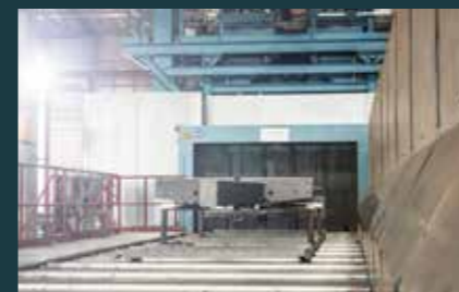
Blasting mechanical pre-treatment for clean and homogeneous surfaces
