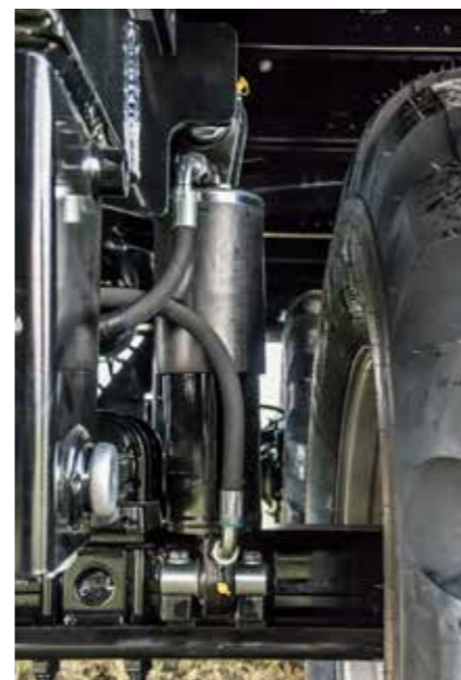
Hydraulic suspension for maximum cornering and slope stability
