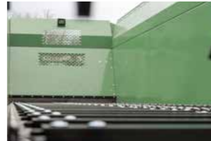
Absolutely smooth trough structure conical towards the rear for easier unloading
