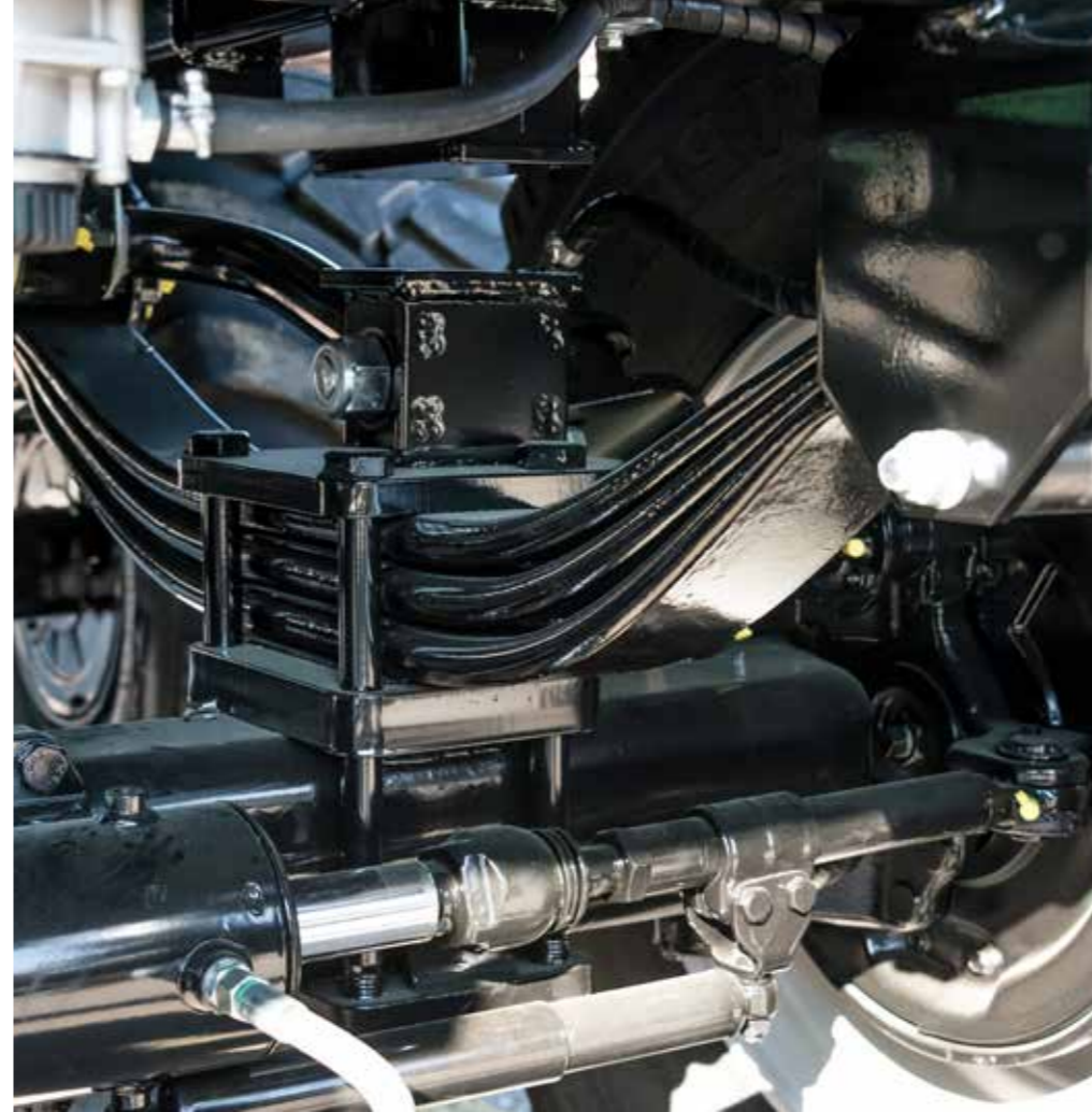
32-ton suspension unit with reinforced balancing rocker
