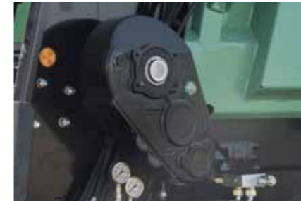
Moving floor drive hydraulically powered via oil bath gear and hydraulic overload protection
