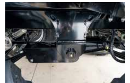
Offset tandem suspension unit adapted for the steering axle, providing better stability and reducing roll tendency
