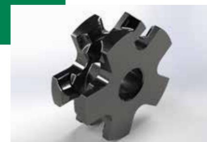
5-star chain wheel used by many competitors (chain angle of approximately 36°)
