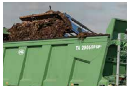
Protection edge During loading, the loading sill is protected from damage by a plastic wear strip
