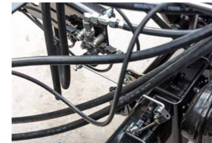
Pneumatic ALB ensures that the braking force is adjusted appropriately
