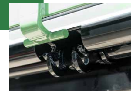
Side hinges from 5 m plateau length with double locking
