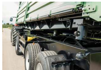
Trapezoidal tilting frame according to truck design with tilting bearings far outboard
