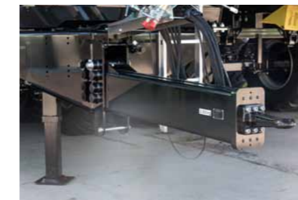
Height-adjustable drawbar manufactured from double-C pressed profiles, as top and bottom coupling
