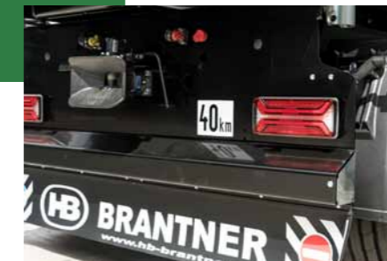
Lighting standard with Agriled full LED rear light with resistor for turn signals
