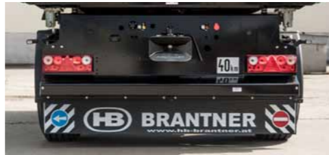
Europoint II lighting with mudguard across the entire width
