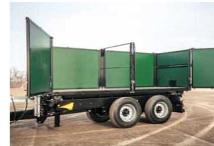
Portal door Standard portal door on the left (optionally also possible on the right), swingably mounted
