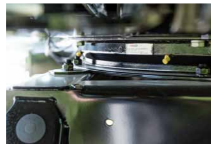
Ball bearing turntable heavy-duty ball bearing turntable from the truck sector
