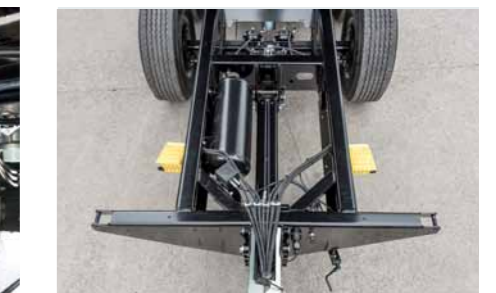
Rectangle frame made of G or double C pressed profiles
