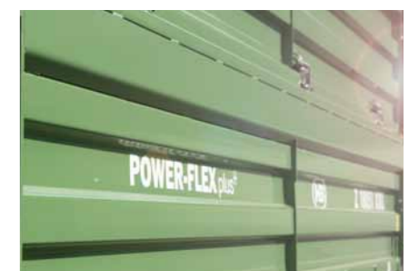
Sideboard stiffening made of 6 mm sheet steel with box profile welded
