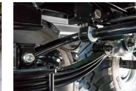
Spring stabilizer optionally available, recommended for steering axles
