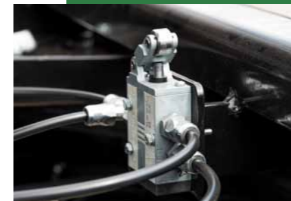
Automatic lowering during the dumping process
