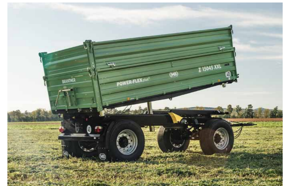
Z 15045 XXL AKTION optional: PROFIL package with 2 tilting cylinders, sideboard stiffening, Sideboard lifting springs and 5 mm sheet steel plate
