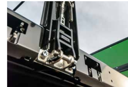
Center post removable without tools - on request helpful when loading boxes or pallets
