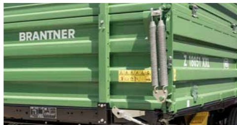
Double side wall lifting spring, rotatable mounted
