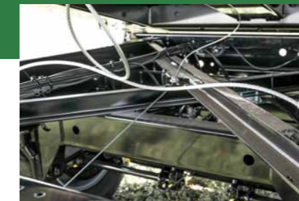
Cross bracing increased torsional rigidity
