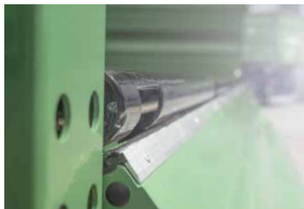
Self-cleaning platform edge edged on all four sides
