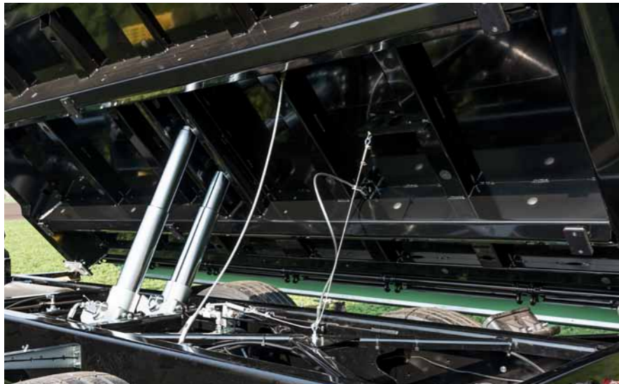
Trapezoidal tilting frame according to truck design including stiffening ribs
