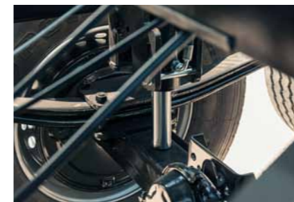
Hydraulic rear axle support standard for optimal suspension comfort
