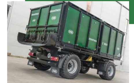
Slide for optimal unloading of sensitive bulk goods (e.g. potatoes)
