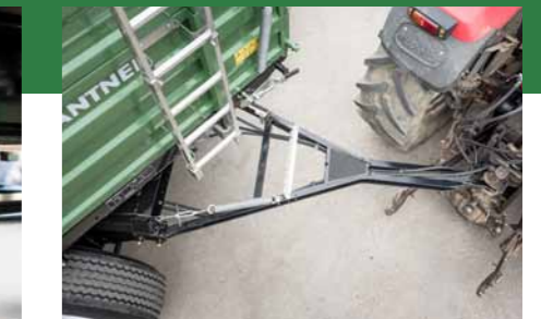
Drawbar Y drawbar for extreme turning radii
