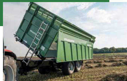
Pendulum wall pendulum-mounted stabilizer walls on the left and right, easy to open
